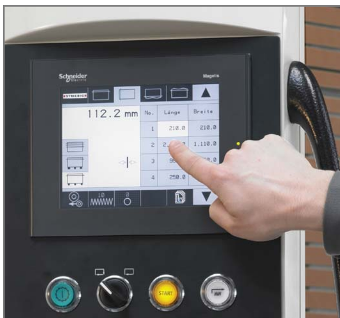
Fig. 6: Just enter the data – that's it. The EPS electronic positioning system fitted to the new CONTROL series allows both cutting axes to be easily positioned to an accuracy of 1/10 mm.
