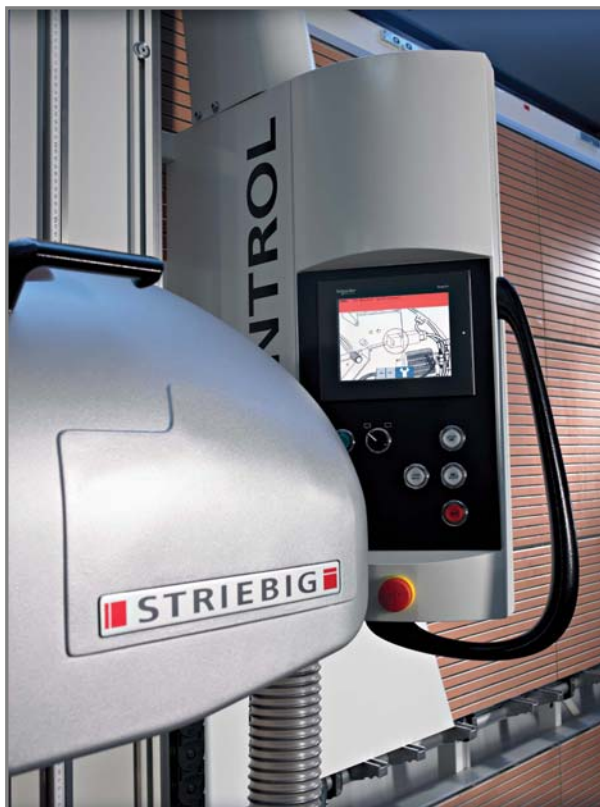
Fig. 5: Using the touch-screen panel fitted to the new CONTROL or EVOLUTION series, the operator can access all of the saw's operating data at any time. Servicing and error messages are visually supported. Communicating with a saw just doesn't get any easier.
