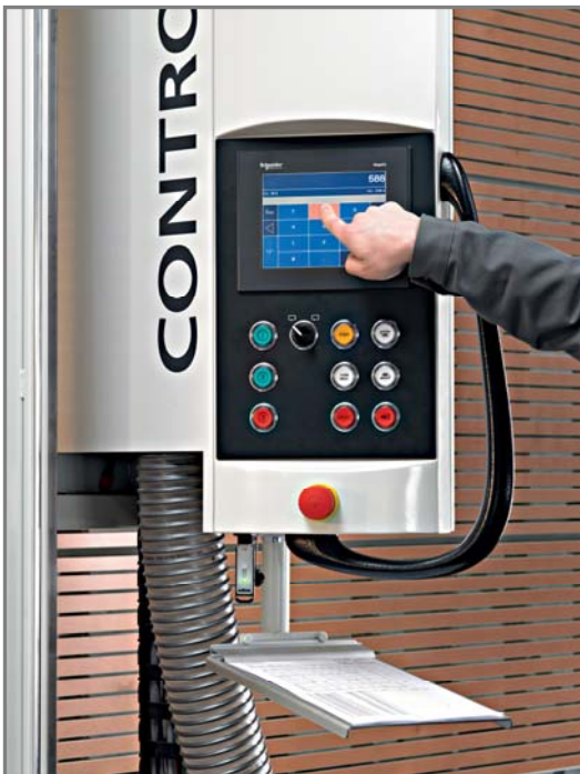
Fig. 2: “Touch & saw” – a touch of the fingertip is all that is required to operate all the functions of the new CONTROL or EVOLUTION series. Multilingual instructions and error detection turn saw operation into child’s play
