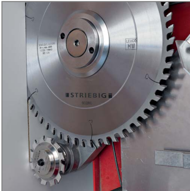
Fig. 8: Saves time, costs and tools – a VSA scoring saw unit decisively extends the service life of a main saw blade.
