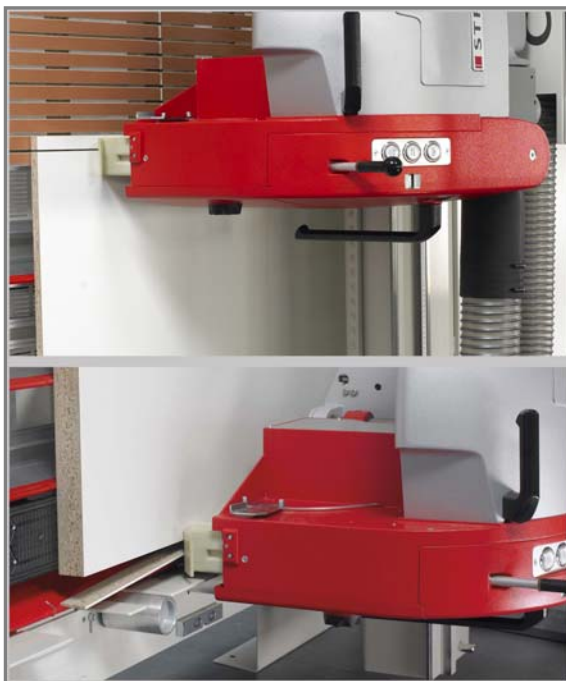
Fig. 4: ABO for automatic upper trimming cuts and the 4SB system for automatic trimming cuts of the lower panel edge. This labour-saving combination is only available on the new CONTROL series.
